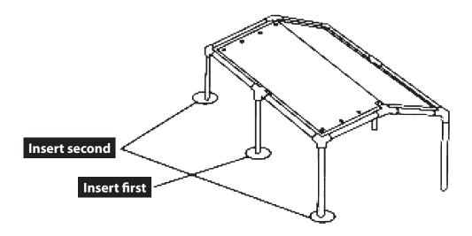
**Step A:** First insert the pipes for the middle poles into the 3- and 4-way connectors, and then connect the end leg pipes in the same way. (See illustration)
